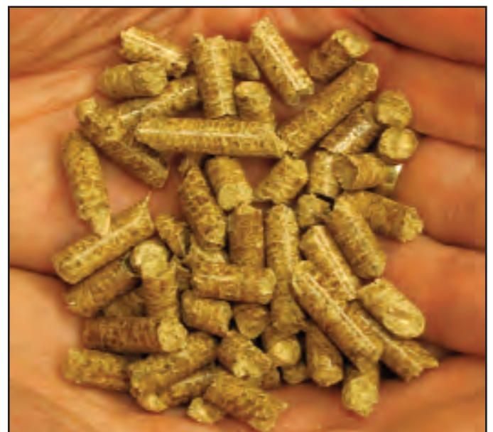
These pellets were made from woody biomass that is formed into an easily transported fuel for utilities or even special home heating stoves.
